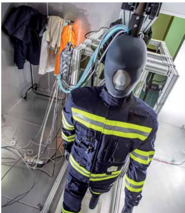
The study of the performance of protective clothing for firefighters using mannequin
