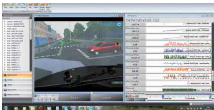
Registration of the track of the sight, vital signs of the driver and technical data from the car
